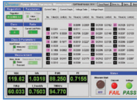
IEC 61000-3-2 Current Harmonics Test (Pre-compliance)
